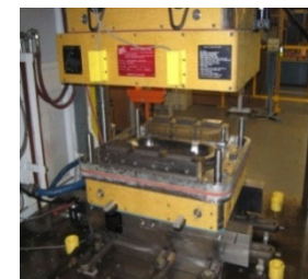
Curing of CFRP
