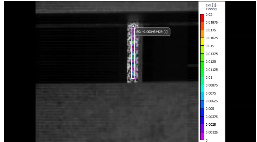
High Rate Tensile Test at ~189 per second (nominal strain rate)*
